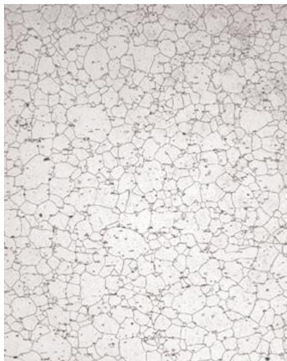
Figure 4. Photomicrograph of INCONEL alloy N06230.
